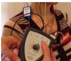
Press the Imp. button and turn the dial fully clockwise.
