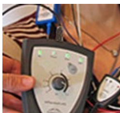
The LED for each electrode will change from red to green as the impedance is found for each electrode.
