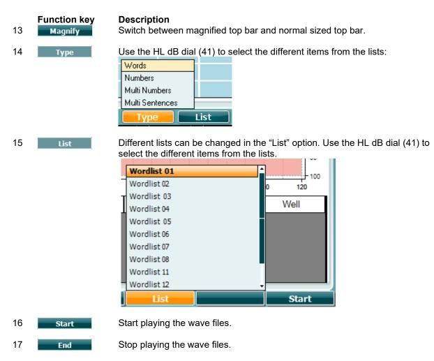
When the Wavefile test is started, the F-buttons will change to recording mode.
