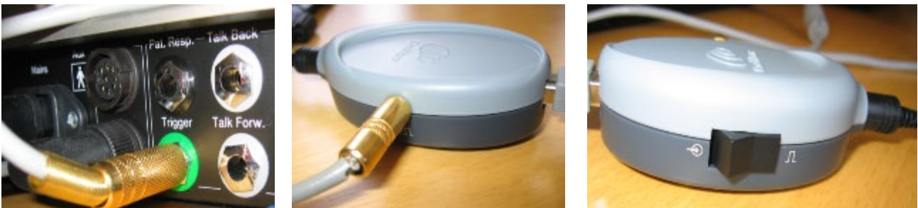
Left: The trigger socket on the back of the Eclipse. Centre and right: The PPS box from Cochlear Nucleus and its settings.
