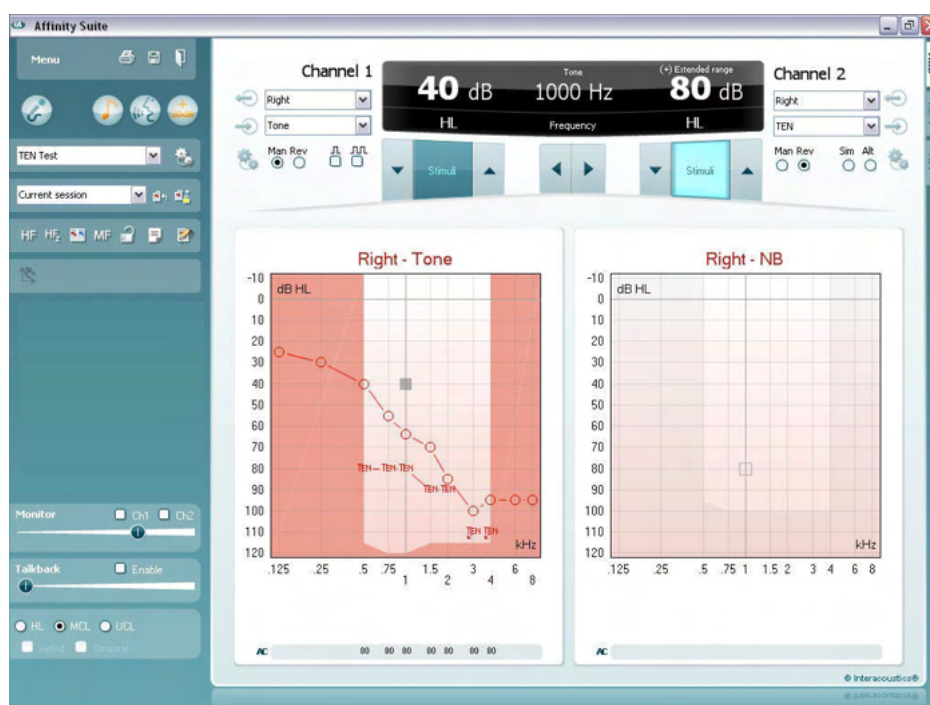
Figure 4. Screen shot from the Callisto™ system. The open circles show the audiometric (absolute) thresholds. The “TEN” symbols show masked thresholds measured for TEN with a level of 80 dB HL. The TEN(HL)-test criteria for a dead region are met at 1.5, 3, and 4 kHz. The result at 2 kHz is inconclusive, as the masked threshold is not 10 dB or more above the audiometric threshold. In such a case, the result at 2 kHz could be checked using a TEN level of 90 dB HL. Overall, the results suggest that this patient has a dead region extending from 1.5 kHz upwards.
